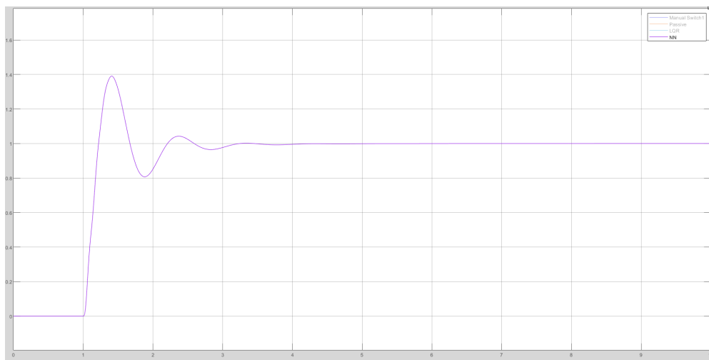
Figure 8: Neural net control response against unit step input (no Gaussian noise)
